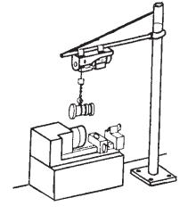
Figure 1. Mounting the Hoist.
